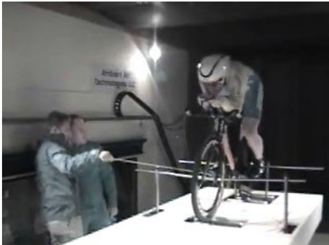
Robby Ketchell and Coach Cummings are using Tufts to see how the air flows over Will and the bike. Will's New Position – It is fast but can he produce power?
